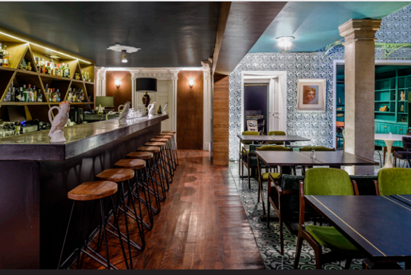
One of the biggest challenges of the construction was to eliminate the load-bearing wall that separated both spaces - the dining area and the bar - by substituting it with a steel beam and columns, now covered with wood.
